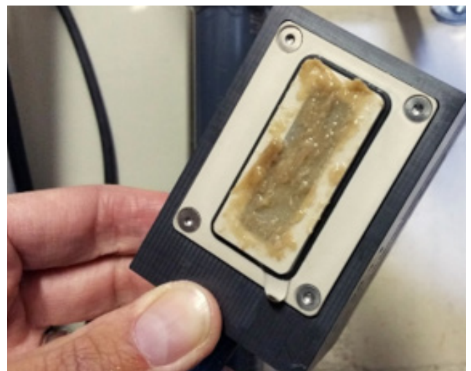
Figure 4 Heated target assembly showing presence of biofilm
